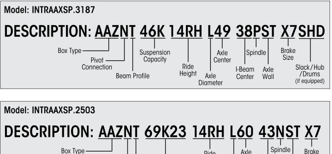
Spindle Box Type Axle Ride Suspension Center Pivot Height Capacity Connection I-Beam Axle Axle **Beam Profile** Center Wall Diameter
